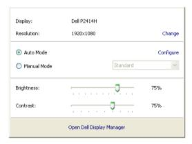
The Quick Settings dialog box also provides access to Dell Display Manager's advanced user interface which is used to adjust Basic functions, configure Auto Mode and access other features.
